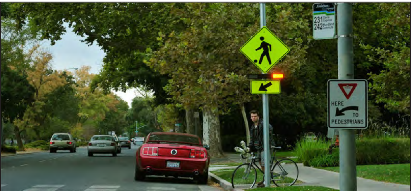
A crossing with flashing warning beacon, such as this example, would increase the safety of pedestrians crossing S. Pittsburgh Street. Flashing beacons can also be installed overhead for even greater visibility.
